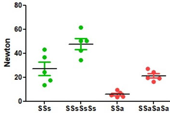
Figure 2: Loop security of 2 and 4 symmetrical sliding half-hitches is 22 and 48N, which is much higher than 2 or 4 asymmetrical ones. (twice  $P < 0.0001$ ). Loop security also increases with the number of half-hitches both for symmetrical and asymmetrical sequences (twice  $P < 0.0001$ ).
